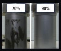
CemPRIME Scrub spacer (right) removes nonaqueous fluid more efficiently compared with a conventional cementing spacer (left).
