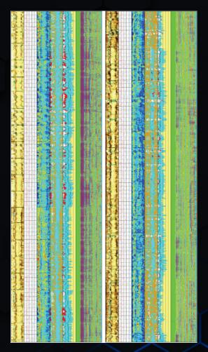
In the conventionally cemented well, left, the cement bond is poor, and uniform, which is common for drilling Fulcrum technology, cement bond is improved, and the higher impedance with texture in places indicates a uniform substance with some mechanical strength.
