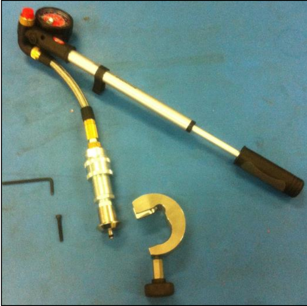
Figure 86 Equipment to apply pressure on the DPG port
