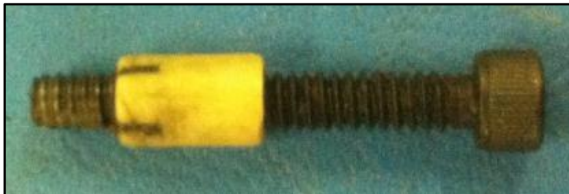
Figure 92 Peek Insert and Soft Tip Screw
