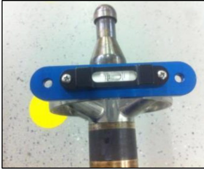
Figure 111 Level to check the High Side
