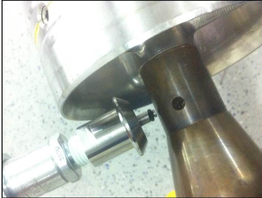
Figure 93 Air Pump adaptor attached to pressure port
