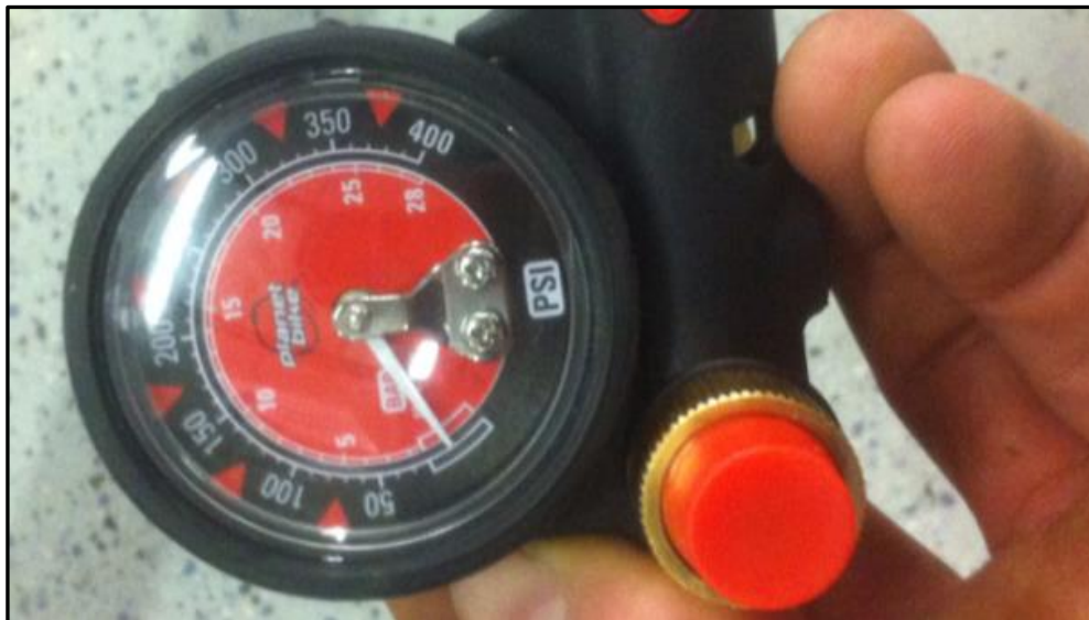
Figure 108 Air Pump Pressure Gauge reading Atmospheric Pressure
