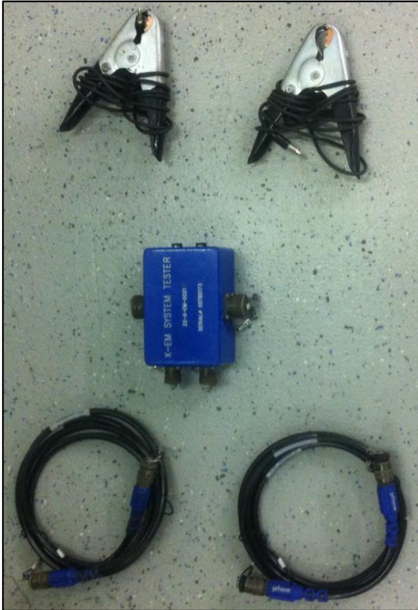
Figure 99 Equipment for Surface test with XEM-RX
