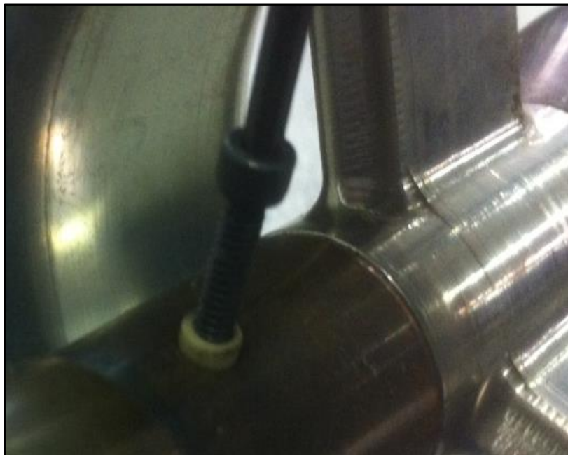
Figure 90 Peek insert being removed
