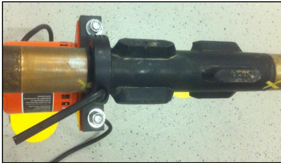
Figure 105 Vibrator Attached to Tool
