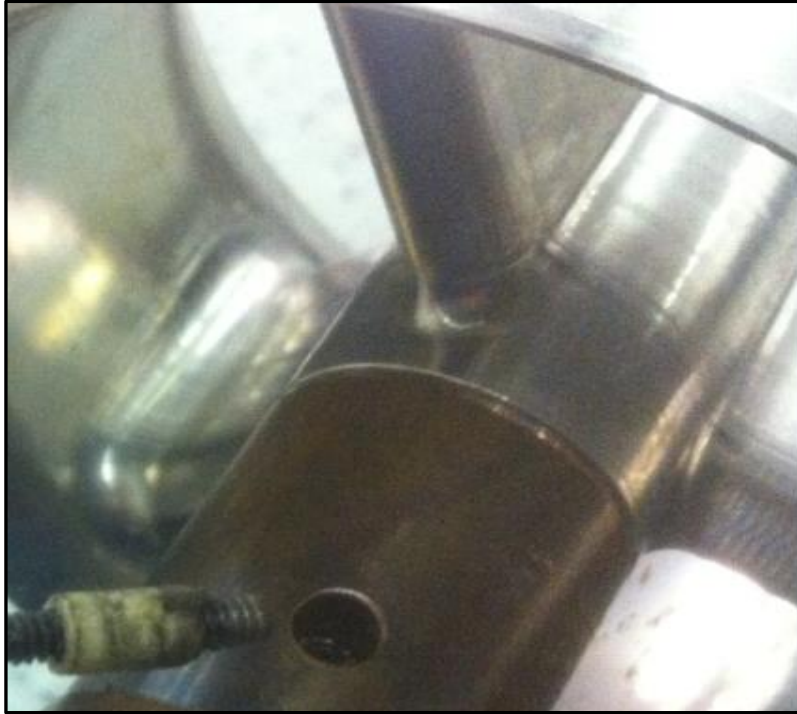
Figure 91 Remove peek insert
