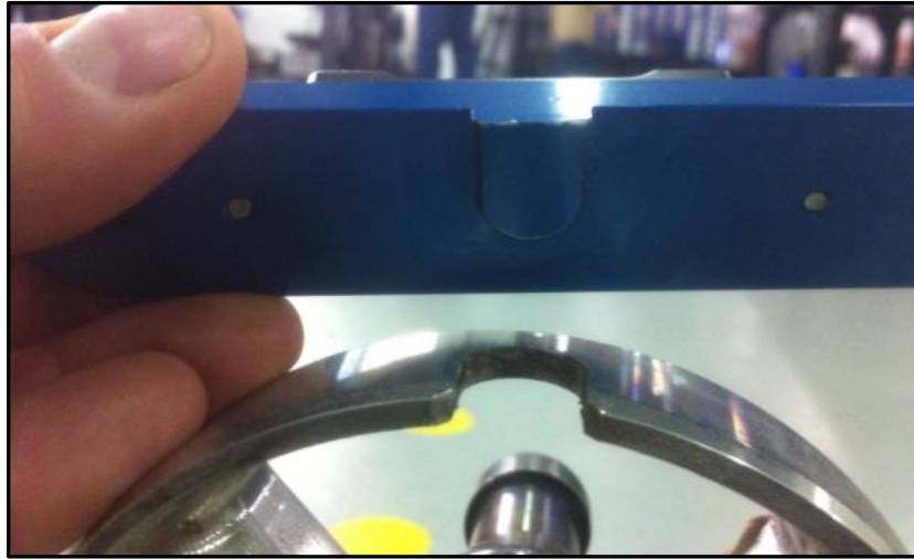
Figure 61 Placing the Level on the spider
