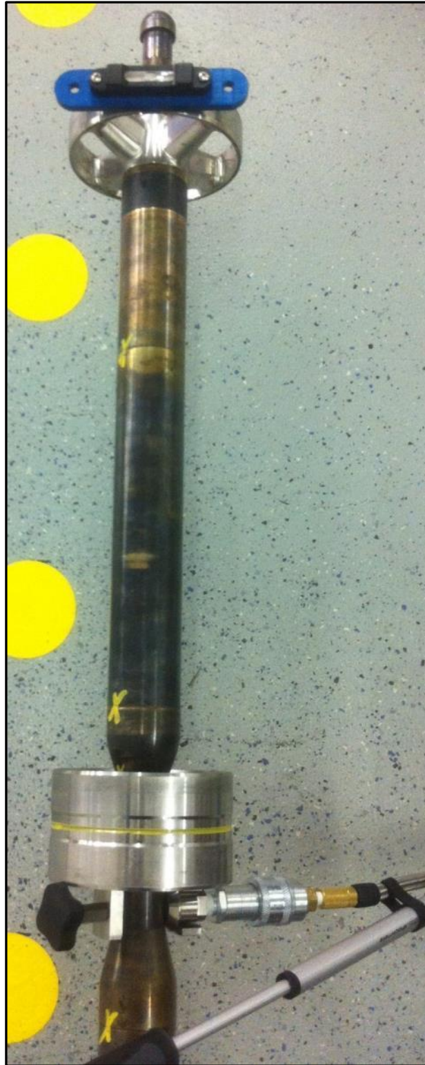
Figure 98 Air pump firmly attached to the DPG probe
