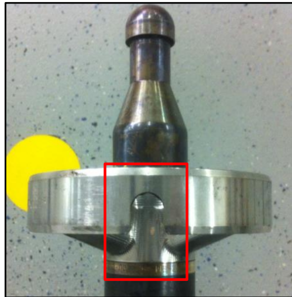
Figure 60 DPG Landing Spider with key slot up
