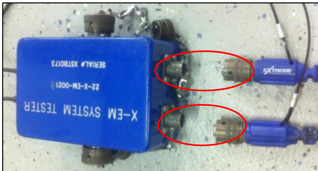
Figure 103 Test cables connected
