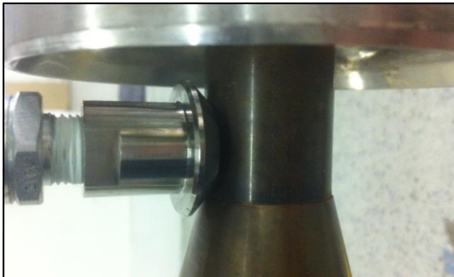
Figure 94 Air pump adaptor attached to port
