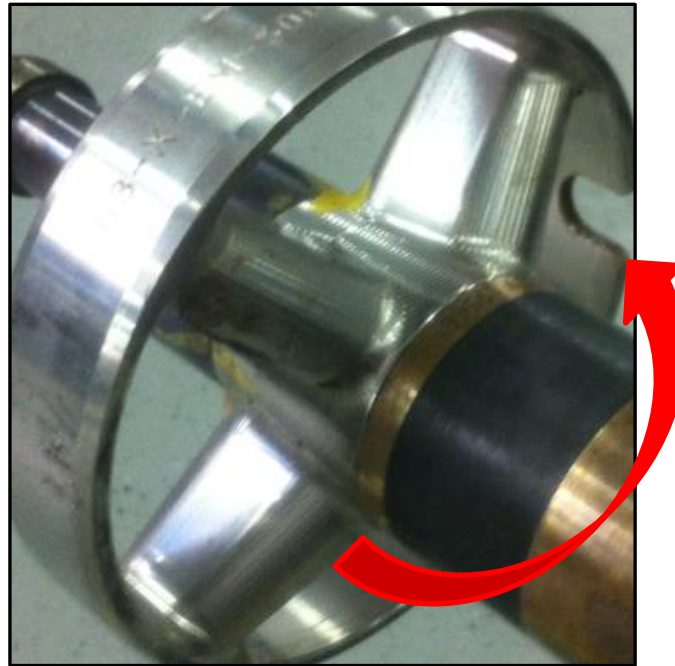
Figure 72 rotate the key slot to 270°
