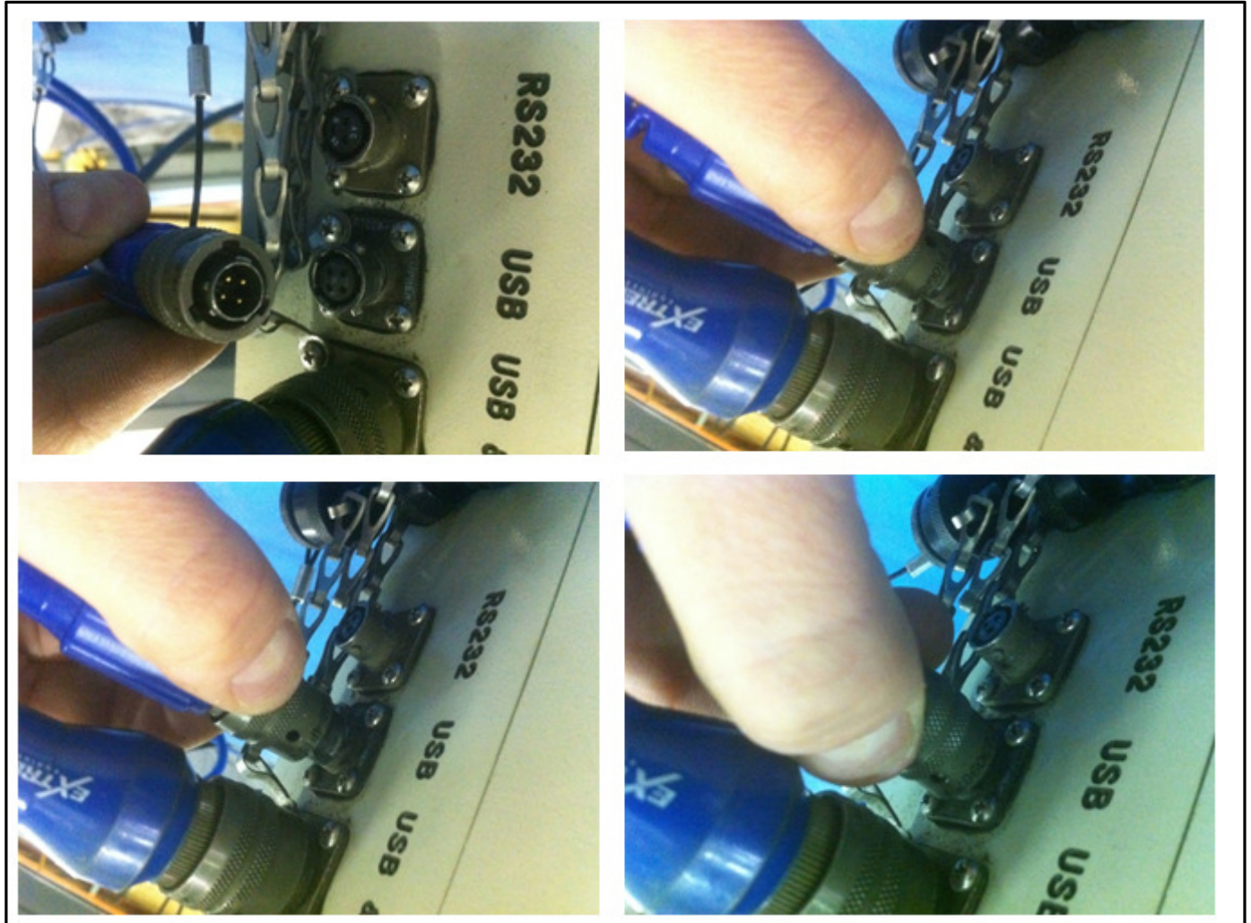
Figure 24 22CABL0049 Connected to Female USB connection on the XRT
