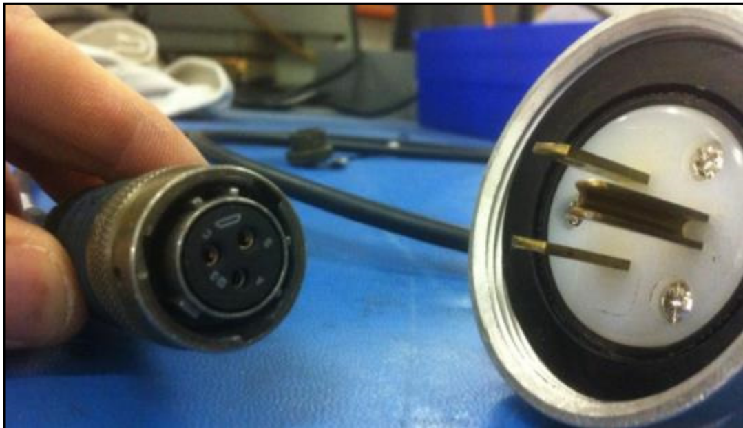
Figure 14 22CABL0037 120V power supply cable
