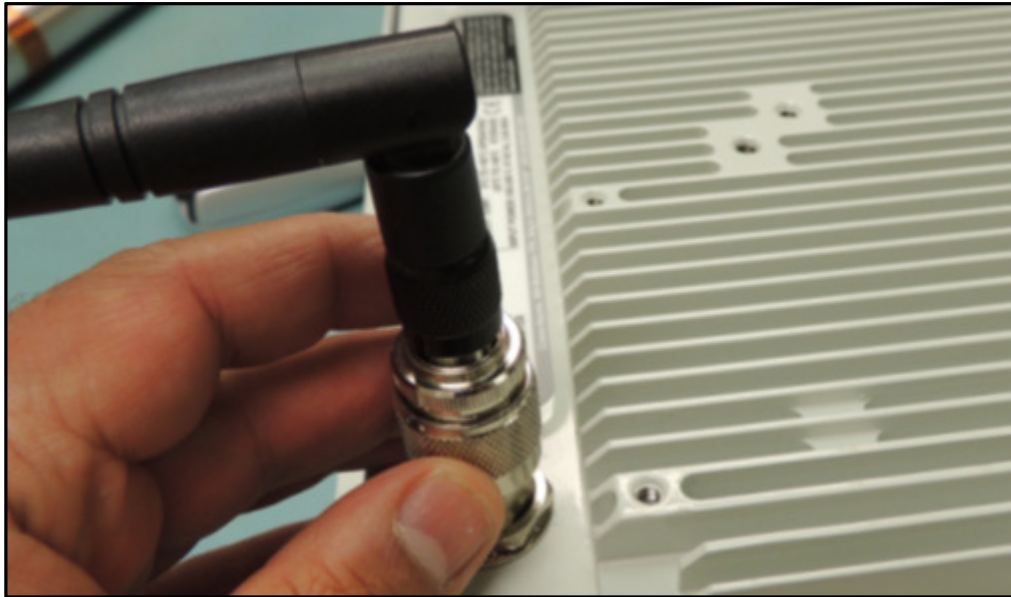
Figure 42 antenna screwed on the antenna Port
