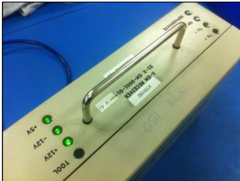
Figure 18 +12V, -12V, +5V LEDs ON, TOOL LED OFF
