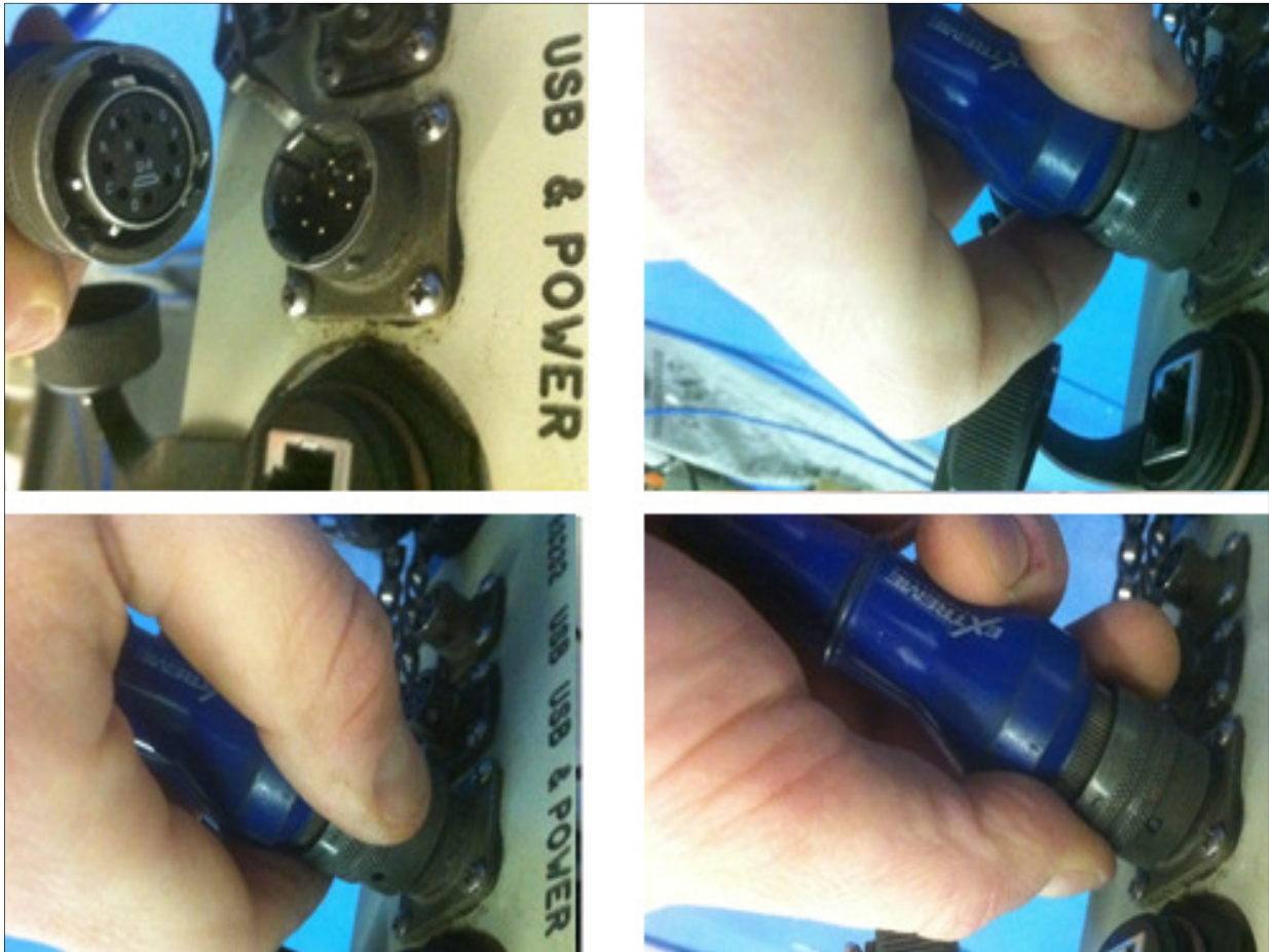
Figure 12 22-CABL-0050 connected with the XRT
