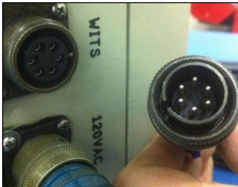
Figure 64 6 x pin Male Connector 22CABL0054
