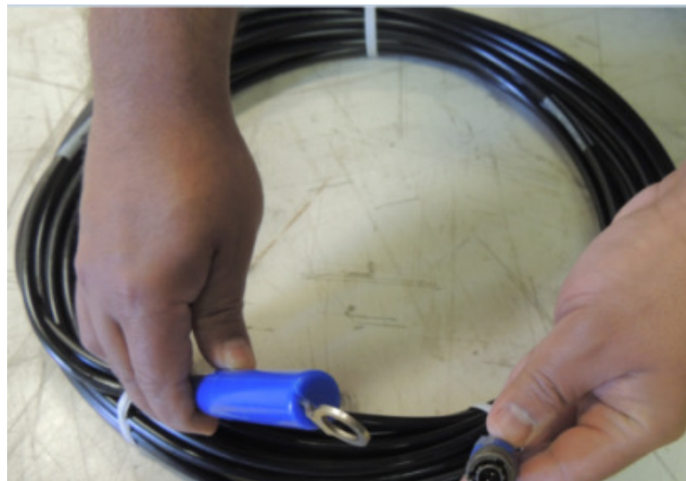
Figure 92 02X-EM0088 Ground stake Cable Clamp
