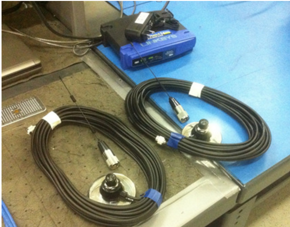
Figure 55 Magnetic base and cables with Antenna
