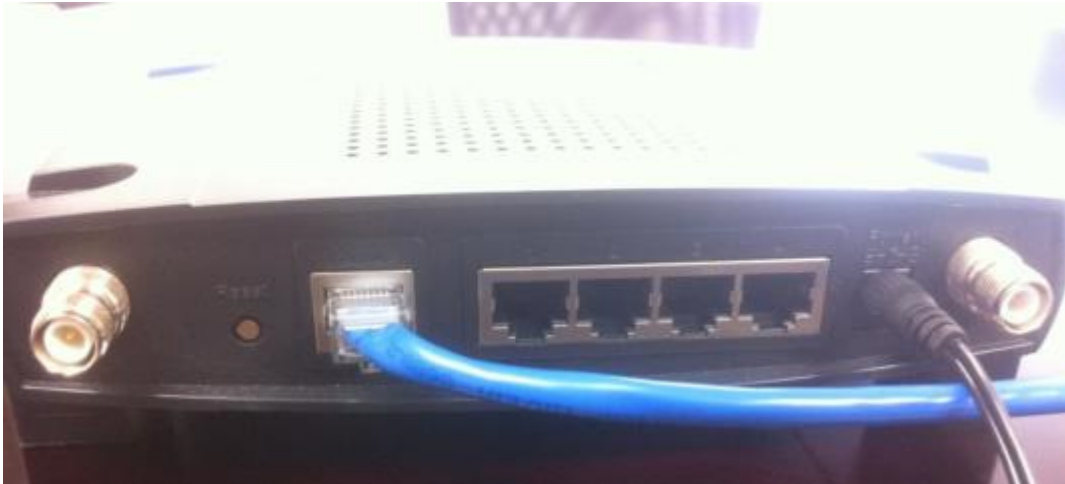
Figure 54 Linksys Router with Ethernet and DC Power Supply Connected
