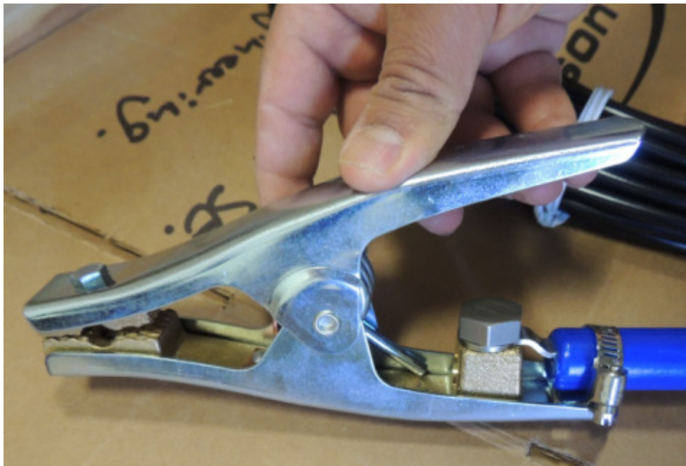
Figure 95 cable secured on to the clamp
