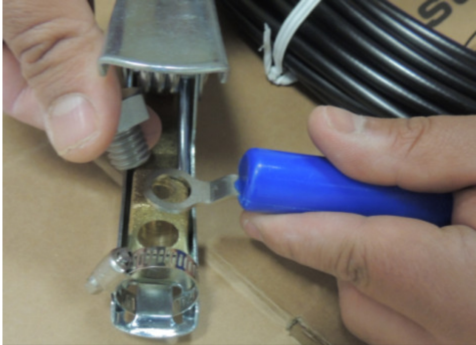
Figure 94 Eye on cable attached with bolt to clamp
