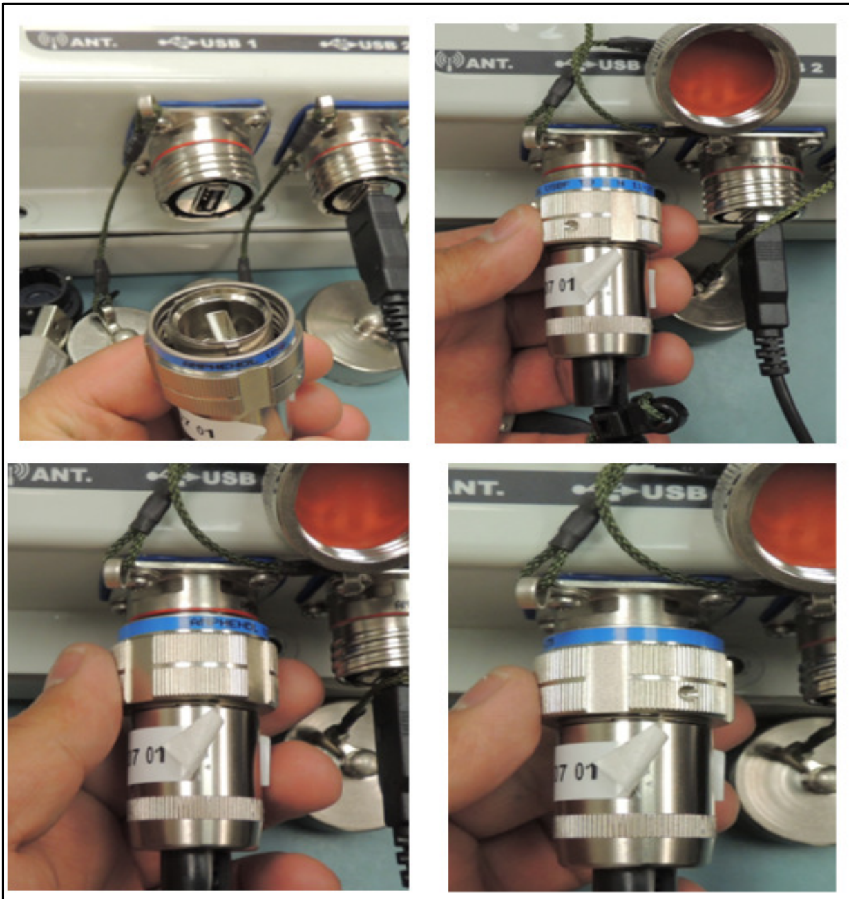
Figure 46 USB Connector on 22CABL0104 connected to USB #1
