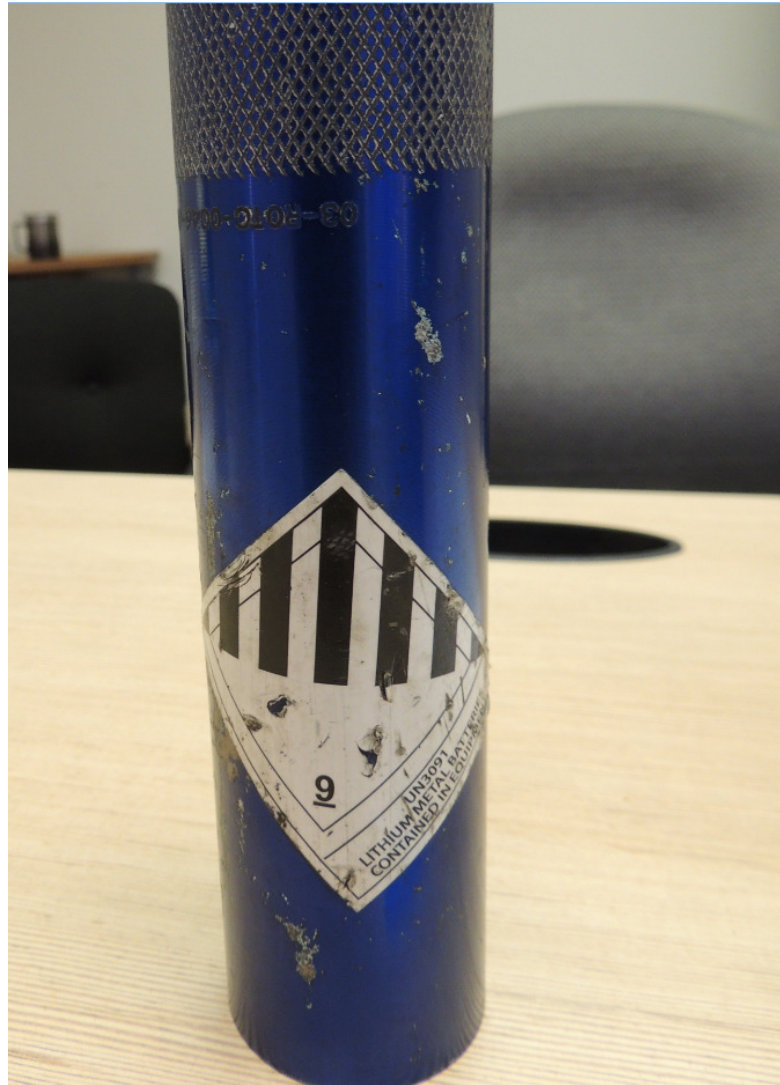
Figure 23 Class-9 Logo UN3091 on Battery dust Cap
