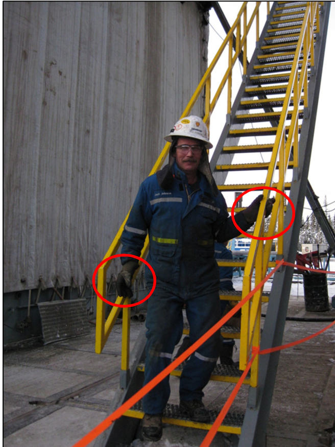
Figure 8 Side stepping while coming down from the rig floor
