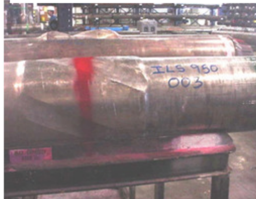
Damaged Insert Bit due to axial shocks
