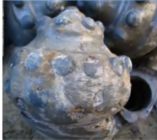
Damaged Insert Bit due to axial shocks
