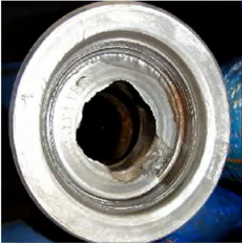
Failure due to fatigue from torsional shocks
