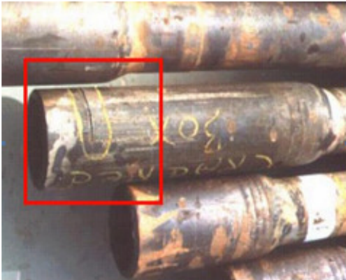
Cracked Drill pipe due to axial shocks
