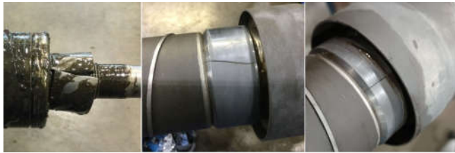
Figure 1. Examples of cracked torquer bearing likely due to transport damage.
